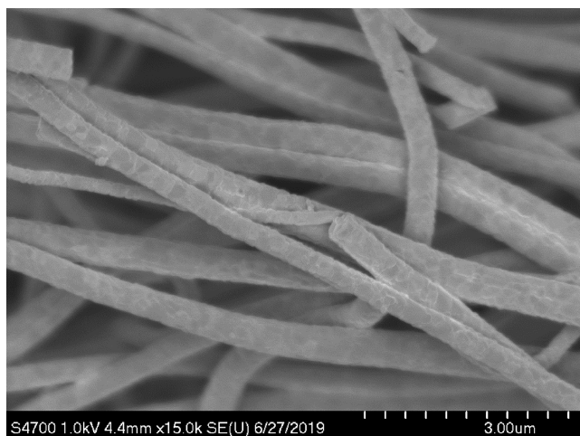
Figure 1. SEM image of raw \text{TiO}_2 nanofibers: i.e., untreated/no Ag. Average diameters are 688 \pm 32 nm, and major dimensions are on the order of tens of micrometers and greater.
