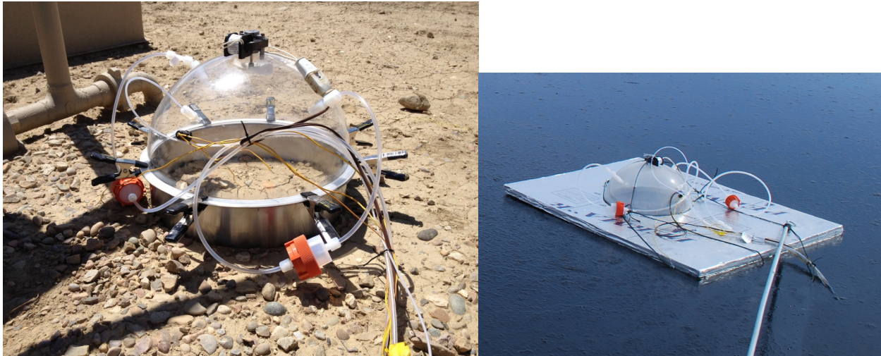
Figure II-1. Field snapshots of our flux chamber. With simple modifications, it can be deployed over soil, water, snow, or ice.
