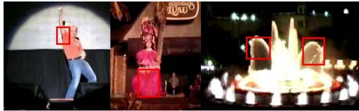
Fig. 8: Three sample frames resulting in the false positives. The red rectangles indicate our misclassified fire regions.
