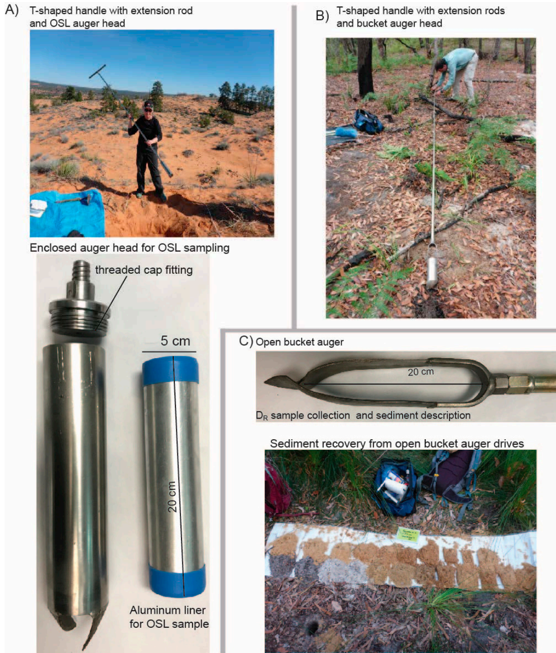
Figure 2. Shallow-sediment auger set-up for luminescence sampling. (A) Optically stimulated luminescence (OSL) auger head with T-shaped handle. The enclosed OSL auger head is fitted with an aluminum liner to contain the OSL sample in a light-proof tube. (B) T-shaped handle with extension rods are used to drive bucket auger. (C) Each drive requires sediment removal from hole, placed on the surface in stratigraphic order (by depth) until desired OSL sampling depth is reached. This material may be needed as part of the D_R sample.
