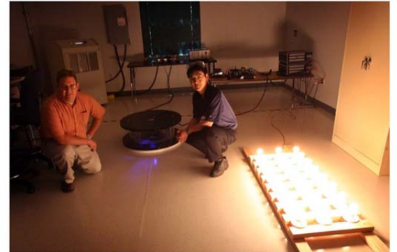
(Leah Hogaten | The Salt Lake Tribune) Utah State University senior electrical engineer Ky Sealy (left) and Dr. Hunter Wu (right) Thursday, July 14 2011 show off the Inductor Charging System that produces 5kw of power. Utah State University's Energy Dynamics Laboratory has developed wireless power transfer technology, which allows charging electrical vehicles without hooking them up to a power source.
