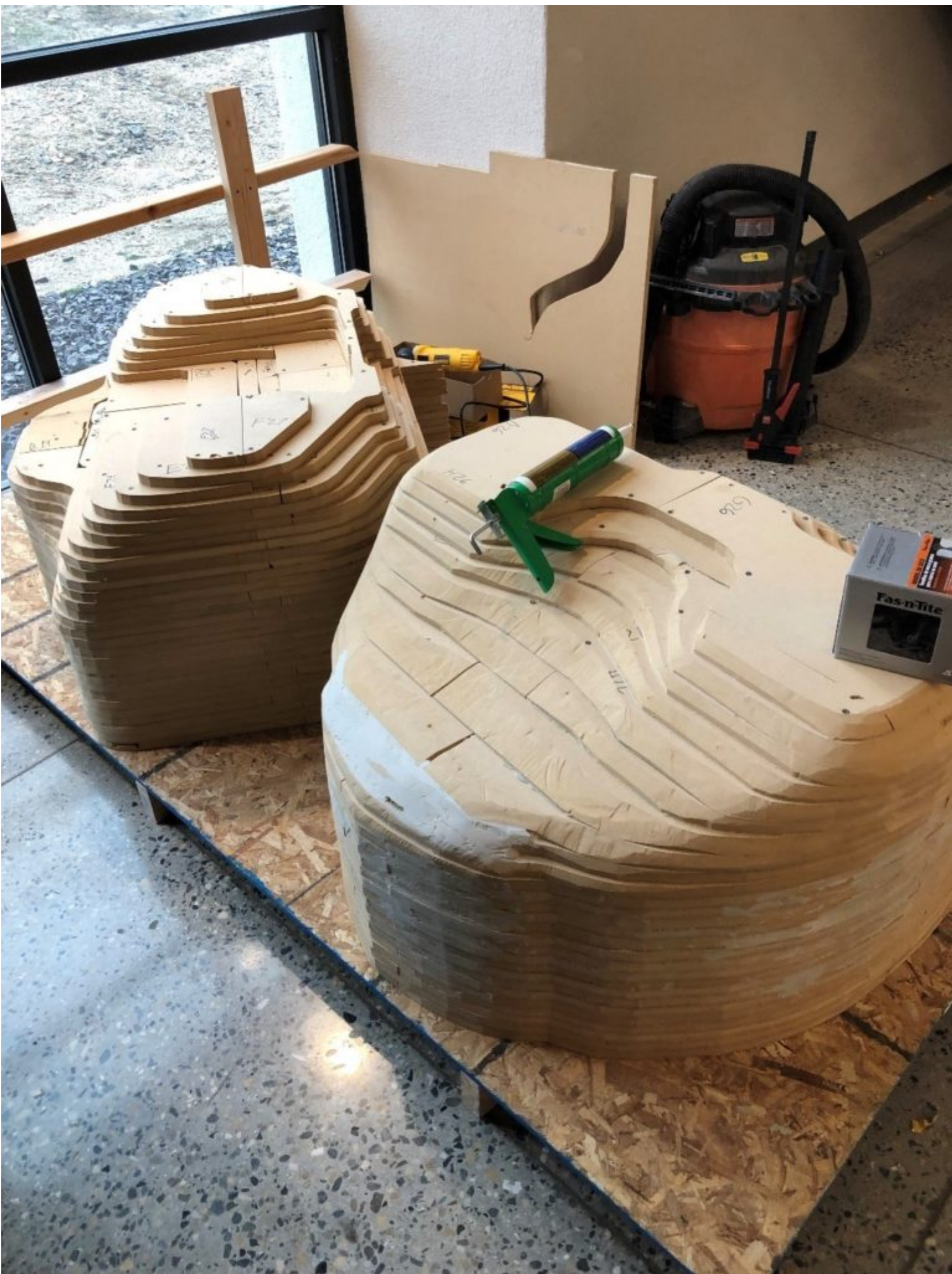
The beginning layer of Bondo applied to the car – some grinding completed. The front portion of the car is in the foreground.
