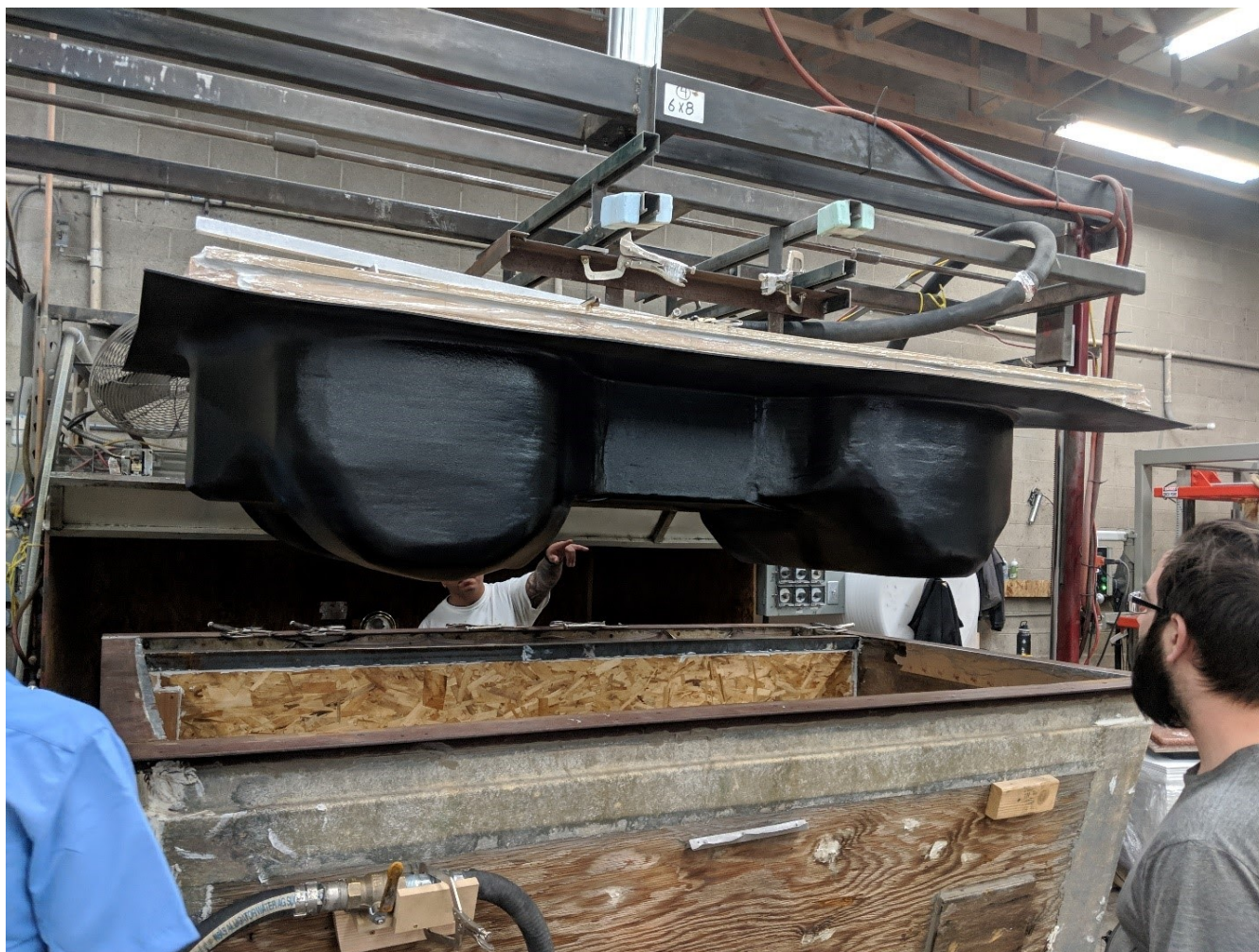
First body coming out of the oven at Magic Vac – the mold is under the ABS (inverted).
